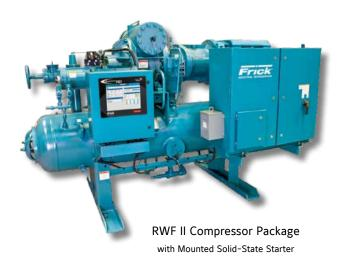
Infinite capacity reduction from 100% to 10% (RWF II) or 25% (RXF) of full load is provided by a slide valve control—one of the most efficient methods of capacity control for screw compressors. Frick compressors allow close system control under widely varying load conditions.
